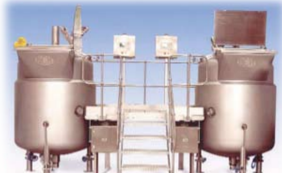
Dual cooking vessel for soup application
